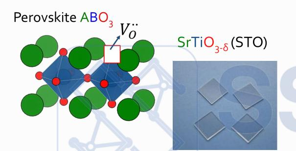
Perovskite ABO<sub>3</sub> structure; Cubic (ideal tolerance factor); ("Si for perovskite oxides")
