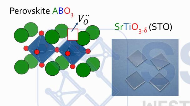
**Note:** even un-doped "pure"  $SrTiO_3$  single crystal contains acceptor dopants such as Mn, Al, Fe, Mg etc. (usually on the level of ~100 ppm, e.g.  $Al'_{Ti}$ ,  $Mg''_{Ti}$ )
