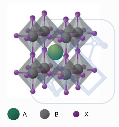
e.g. Methylammonium lead iodide CH<sub>3</sub>NH<sub>3</sub>PbI<sub>3</sub> (MAPbI<sub>3</sub>)
