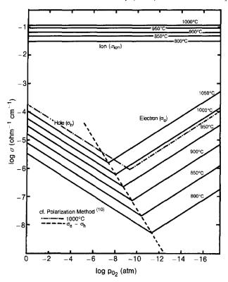
**Figure 2** Electronic and ionic conductivity of 8YSZ (Park *et al.*, *J. Electrochem. Soc.*, **136**(10) 2867 (1989)).
