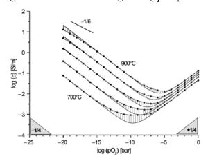
Figure 1  $\log \sigma \sim \log pO_2$  plot of acceptor-doped SrTiO<sub>3</sub> single crystal (Ohly *et al., J. Am. Ceram. Soc.*, **89**(9) 2845–2852 (2006)).
