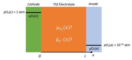
Figure 3 Schematic of a model solid oxide fuel cell with YSZ as
