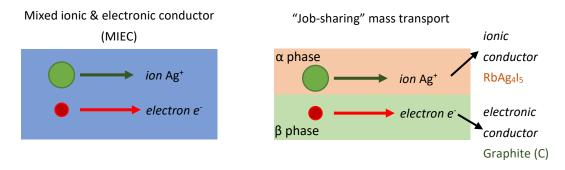
Figure 1 Chemical diffusion in MIEC and job-sharing composites.
