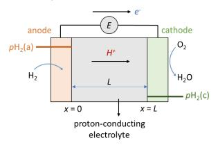
The working principle of such a fuel cell can be shown as the figure above. The proton-conducting electrolyte is sandwiched between an anode and a cathode. Consider the open-circuit condition with  $pH_2(a)$  and  $pH_2(c)$  as the (effective) hydrogen partial pressure at the anodic and cathodic side, respectively.
